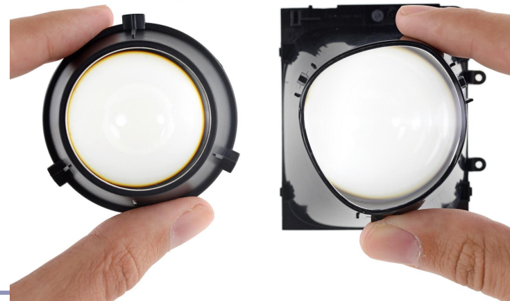
Teardown of an Oculus Rift CV1 showing details of lenses and displays https://www.ifixit.com/Teardown/Oculus+Rift+CV1+Teardown/60612
